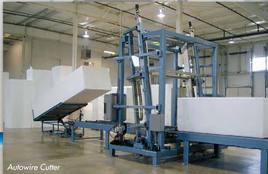
CNC Contour (Shaping/Cutting) Parts up to 110" profile, table length 200"
